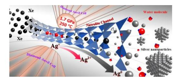
The Lawrence Livermore team used a high pressure diamond anvil cell to show that under high pressure and temperature, a silicate mineral, made up mostly of silver, irreversibly inserts xenon into its micropores and undergoes charge separation This mineral absorbs and retains significant amounts of xenon at conditions found in the subsurface of Earth.
