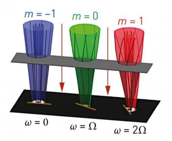
A transmission electron microscope creates beams of electrons with different vortex properties (m) that are focused on an observational plane (black) by a magnetic field (red arrows). A plane (gray) is used to cut off parts of the electron beam to analyze electron trajectories with different angular rates ( $\omega$ ). Credit: Modified from Ref. 1 and licensed under CC BY 4.0 © 2014 P. Schattschneider et al.
