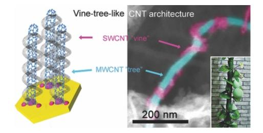
Hierarchical vine-tree-like carbon nanotube architectures composed of vine-like single-walled carbon nanotubes wrapping around the tree-like multi-walled carbon nanotubes are fabricated through in-situ chemical vapor deposition self-assembly. The vine-tree-like nanoarchitectures exhibit excellent cycling stability and rate performance when employed as the cathode scaffolds for lithium-sulfur batteries.
