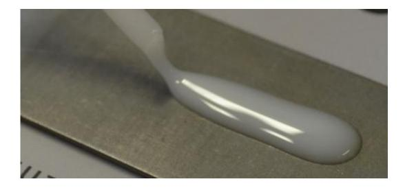
The variable elasticity offered by dual-cure adhesives provides significantly longer-lasting adhesive bonds. Credit: Fraunhofer LBF
