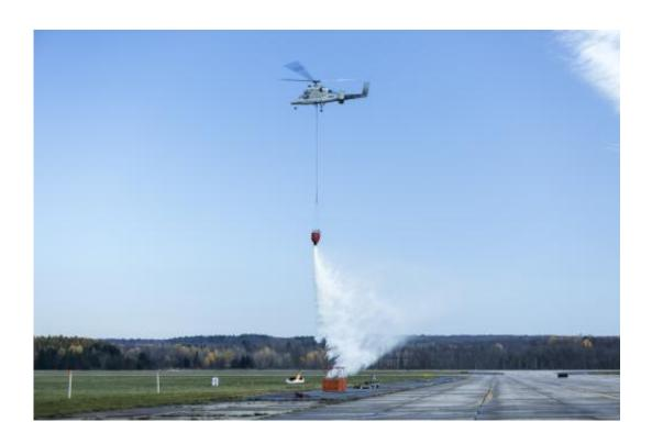
The unmanned K-MAX, helicopter successfully conducted a firefighting mission during a demonstration on Nov. 6. Aided by the small unmanned Indago quad rotor, unmanned K-MAX extinguished several fires while collecting and dropping more than 24,000 pounds of water onto the flames in one hour.
