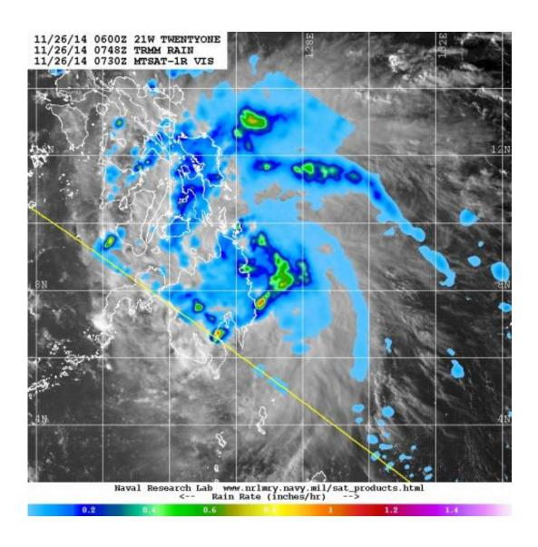
On Nov. 26, the TRMM satellite revealed areas of heavy rainfall in fragmented bands east of the center of circulation, where rain was falling at more than 1 inch (25 mm) per hour (red). Japan's MTSAT-1 satellite provided cloud data. Credit: NASA/NRL
