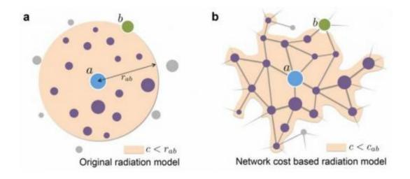
These diagrams depict the widely used "radiation" model used to analyze traffic flows (a) and the modified version (b) used by this research team, which adds a measure of the "cost" (in this case, time spent) of each possible route between two locations. That model is then used to compute average traffic flows through a wider system of highways, as depicted in the first image.
