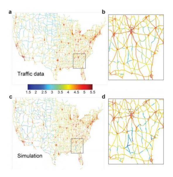
Actual data on traffic times through the U.S. highway system (a) and a closeup view of one region (b) are compared with comparable data obtained through the simulation system devised by the researchers (c and d), showing a good agreement between the two.
