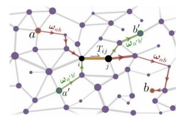
This diagram shows how researchers compute average traffic flows through a wider system of highways.
