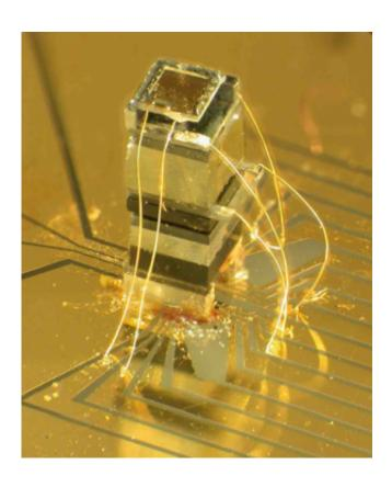
The NIST chip-scale magnetometer. The sensor is about as tall as a grain of rice. The widest block near the top of the device is an enclosed, transparent cell that holds a vapor of rubidium atoms.
