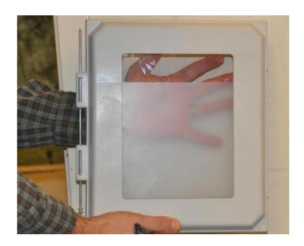
A year's worth of sandblasting by intense Antarctic winds rendered the window of a camera mount almost opaque. The clear portion had been covered by an anchor strap.
