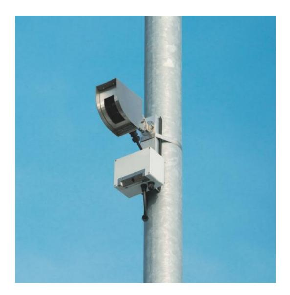
A vehicle measurement sensor at a roadside rest stop.
