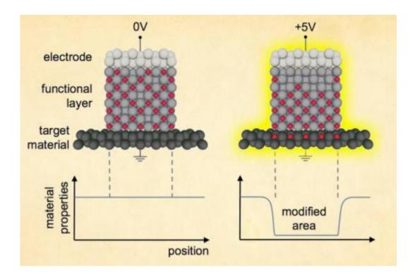
This diagram shows the principle behind using voltage to change material properties. In this sandwich of materials, applying a voltage results in movement of ions — electrically charged atoms — from the middle, functional layer of material into the target layer. This modifies some of the properties — magnetic, thermal, or optical — of the target material, and the changes remain after the voltage is removed. Credit: Diagram courtesy of the researchers; edited by Jose-Luis Olivares/MIT
