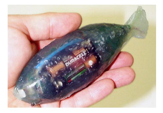
Pacific Northwest National Laboratory scientists have developed an electronic sensor fish that is designed to record some of the environmental conditions fish may encounter while passing through hydropower turbines. The original six-inch rubbery fish (pictured) has since been revised into the form of a 3.6-inch plastic tube.
