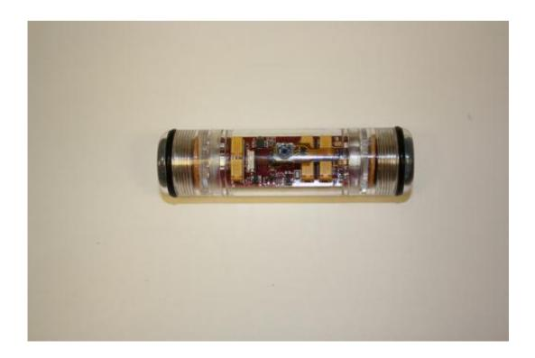
PNNL's improved Sensor Fish is a small tubular device filled with sensors that analyze the physical stresses fish experience as they pass through dams and other hydropower structures. The device's latest version costs about 80 percent less and can be used in more hydro structures than its predecessor, according to a paper published in the journal Review of Scientific Instruments.
