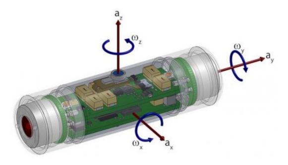
A technical drawing of the latest version of the Sensor Fish, illustrating the various directions in which the device's motions are recorded.
