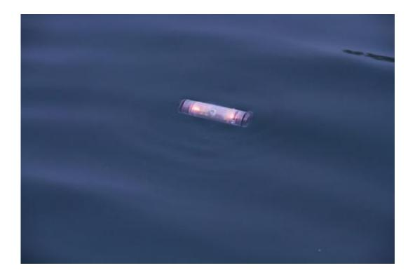
The latest version of PNNL's Sensor Fish floats in water and flashes its LED lights after a test. LED lights help researchers see and retrieve the device.
