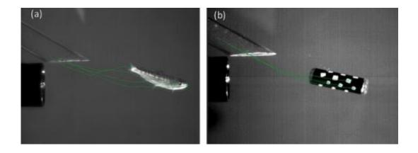
A live juvenile fish (left) and the previous version of the Sensor Fish (right) are shown side-by-side as they're exposed to a simulated dam turbine environment. This test helped PNNL researchers correlate the injuries some fish experience with the Sensor Fish's measurements.
