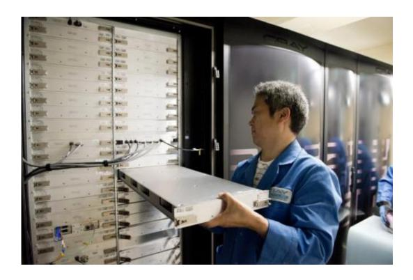
A staff member of the Cray Japan Inc. exchanging a blade. 266 blades for calculations were replaced. Credit: NAOJ
