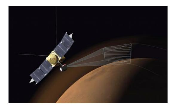
MAVEN's Ultraviolet Imaging Spectrograph (IUVS) uses limb scans to map the chemical makeup and vertical structure across Mars' upper atmosphere. It detected strong enhancements of magnesium and iron from ablating incandescing dust from Comet Siding Spring. Credit: NASA
