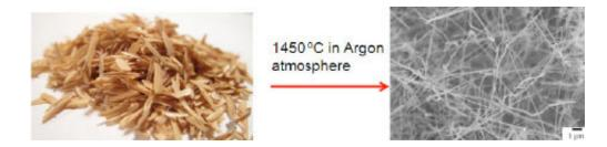
For U.S. Naval Research Laboratory scientists, the conversion of rice husks to high value SiC nanowires may provide new materials for electronic and structural applications. Credit: U.S. Naval Research Laboratory
