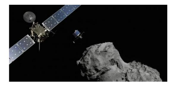
Rosetta deploys the Philae lander to comet 67P/Churyumov–Gerasimenko. ESA/ATG medialab; Credit: ESA/Rosetta/Navcam
