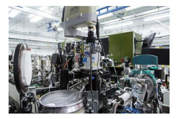
Equipment used in a highly automated X-ray crystallography system at SLAC's Linac Coherent Light Source X-ray laser. The metal drum at lower left contains liquid nitrogen for cooling crystallized samples studied with LCLS's intense X-ray pulses. Credit: SLAC National Accelerator Laboratory
