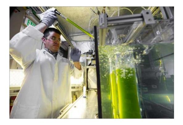
NREL Research Technician Nick Sweeney inoculates algae being grown in a tent reactor. Algae brought back to active states from cryogenic tanks need aerobic environments to meet their full potential as biofuels. Credit: Dennis Schroeder, NREL
