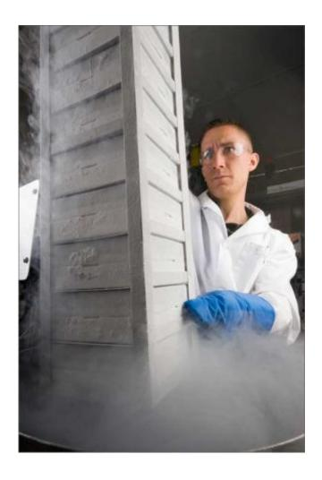
An NREL researcher removes boxes of algae cultures from a cryopreservation tank. The tank is cooled using liquid nitrogen, which freezes and preserves the algae cultures. NREL researchers are studying algae as a potential source of biofuels. Credit: Pat Corkery
