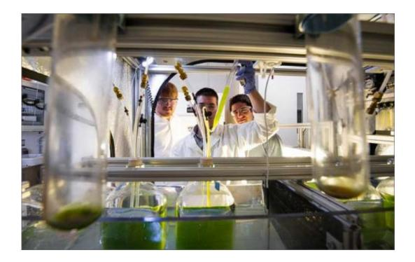
Robert Sebag and Will Long watch Nick Sweeney, center, inoculate algae being grown in a tent reactor. The reactor, developed at NREL, controls light, carbon dioxide delivery, and temperature to establish baseline growth curves and recreate real-world growth conditions, allowing researchers to grow denser cultures in less time. Credit: Dennis Schroeder, NREL
