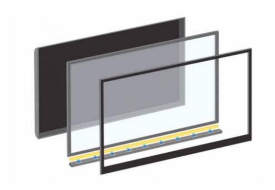
Manufacturers implement the Color IQ component (shown here as a thin, yellow bar) into their televisions during the normal construction process, but use blue LEDs (blue dots) in place of the standard white LED back lights. Credit: QD Vision
