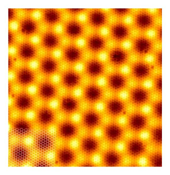
Scanning tunnelling microscopy (STM) image of graphene on Ir(111). The image size is  $15 \text{ nm} \times 15 \text{ nm}$ . Credit: ESRF
