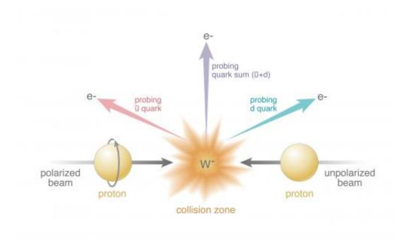
Collisions of polarized protons (beam entering from left) and unpolarized protons (right) result in the production of W bosons (in this case, W-). RHIC's detectors identify the particles emitted as the W bosons decay (in this case, electrons, e-) and the angles at which they emerge. The colored arrows represent different possible directions, which probe how different quark flavors (e.g., "anti-up," u and "down," d) contribute to the proton spin.
