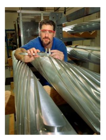
Specialized accelerator magnets known as Siberian snakes have a corkscrew design that helps maintain the polarization of proton beams for RHIC experiments. Keeping all the proton spins aligned in a given direction within at least one of RHIC's colliding beams helps scientists tease out the spin contributions of the proton's internal components.
