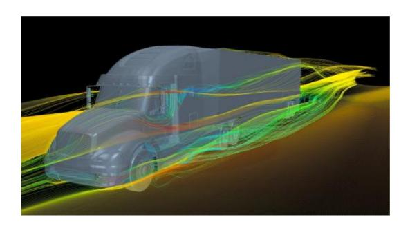
The computational images represent a single flow simulation around a typical onthe-road heavy vehicle at highway speed from different viewpoints. In this simulation, the trailer is aerodynamically treated by skirts and a tail fairing. The simulation incorporates a full-scale high-fidelity truck model with moving wheels. The flow field around the vehicle is highlighted by streamlines which are colored by velocity magnitude.
