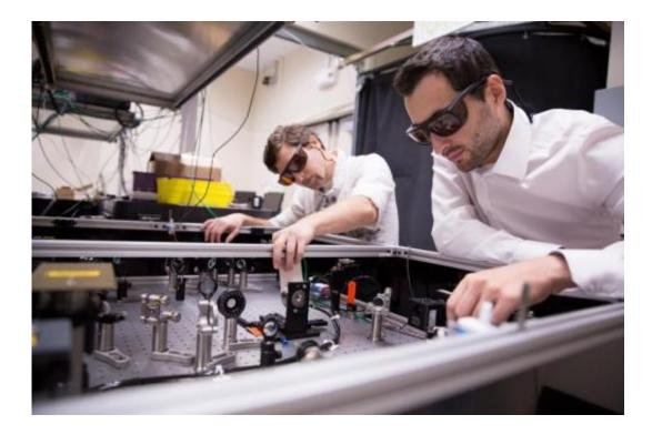
SLAC researchers Michael Litos, left, and Sebastien Corde use a laser table at the Facility for Advanced Accelerator Experimental Tests (FACET) to create a plasma used for accelerating electrons to high energies in a very short distance. Credit: SLAC National Accelerator Laboratory
