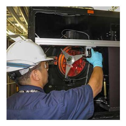
Target Area Operator Mike Visaya aligns a VISAR transport mirror in preparation for an experiment.
