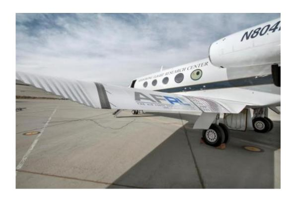
For taxi testing on Oct. 31, 2014 at NASA's Armstrong Flight Research Center at Edwards Air Force Base, in California, the Adaptive Compliant Trailing Edge (ACTE) flap was extended to 20 degrees deflection. Flight results will validate whether the seamless design with its advanced lightweight materials can reduce wing structural weight, improve fuel economy and efficiency, and reduce environmental impacts. Credit: NASA/Ken Ulbrich
