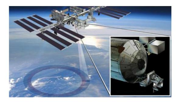
ISS-RapidScat instrument, shown in this artist's rendering, was launched to the International Space Station aboard the SpaceX CRS-4 mission on Sept. 21, 2014 and attached at ESA's Columbus module. It will measure ocean surface wind speed and direction and help improve weather forecasts, including hurricane monitoring. Credit: NASA/JPL-Caltech/Johnson Space Center.
