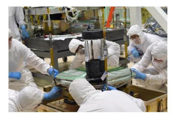
Engineers and technicians check the fit of ICESat-2's telescope to its sling, before moving it into place on the instrument's optical bench. Credit: Debbie McCallum/NASA
