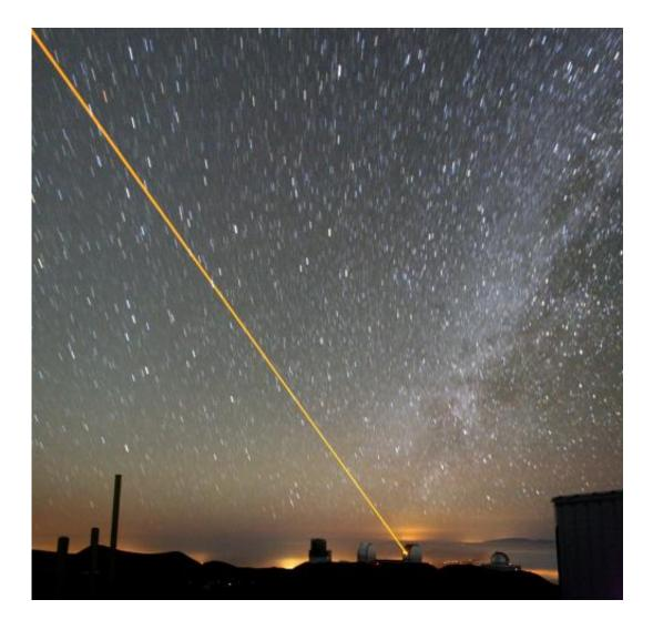
The twin telescopes at Keck located on the summit of Mauna Kea in Hawaii. Each having 10-meter mirrors, they are currently the largest telescopes. The laser beam acts as an artificial guide star (shown in the picture) to correct for the blurring due to atmospheric disturbances, a technique known as adaptive optics for high-resolution observations. Credit: Paul Hirst
