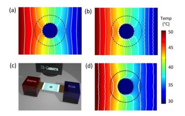
Simulations of heat flux cloaking, one function of the multiphysics cloak. In (c), the heat-transfer measurement set-up involves hot and cold water tanks and an infrared camera to capture the temperature field through thermal radiation emission. Credit: Ma, et al. ©2014 American Physical Society
