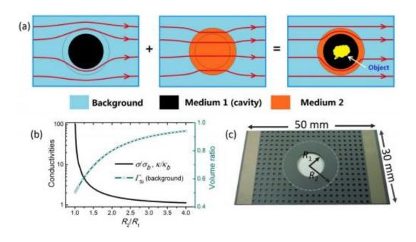
(a) The bifunctional cloak consists of an empty cavity (black) that scatters current and heat flow, along with an outer solid medium (orange) that concentrates current and heat flow. (b) Electric and thermal conductivities as a function of the inner:outer radius ratio of the cloaking shell. (c) A photograph of the cloak. Credit: Ma, et al. ©2014 American Physical Society
