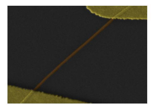
A titanium oxide nanowire acts as both a diode and a memristor
