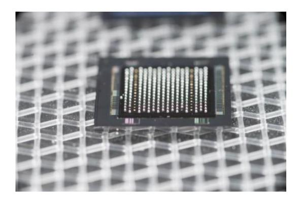
The 64-by-64 pixel VIPIC prototype, pictured with a sensor on the bottom and solder bump-bonding bump on top, ready to be received on the printed circuit board. Credit: Reidar Hahn
