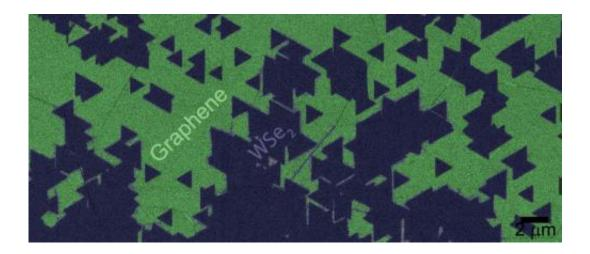
Colorized TEM image of tungsten disulfide triangles (black) growing on graphene substrate (green). Credit: Pennsylvania State University
