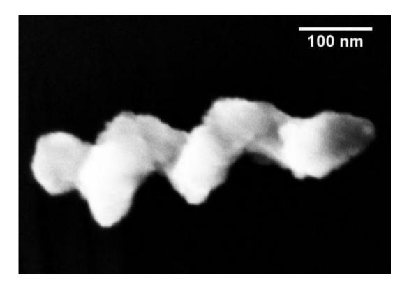
Propeller-driven nano-submarine: The researchers in Stuttgart incorporated a magnetic material in the tiny propeller and spun it by applying a rotating magnetic field so that it rotates and thus drills its way through a liquid. Credit: Debora Schamel / MPI for Intelligent Systems
