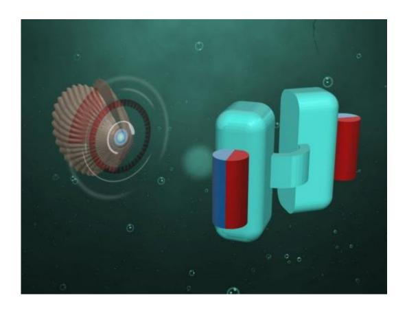
Planck researchers in Stuttgart has built a tiny submarine, shown in the drawing on the right. Small magnets, shown here as red and blue cylinders, open and close the two halves (shells) of the device. Credit: Alejandro Posada / MPI for Intelligent Systems
