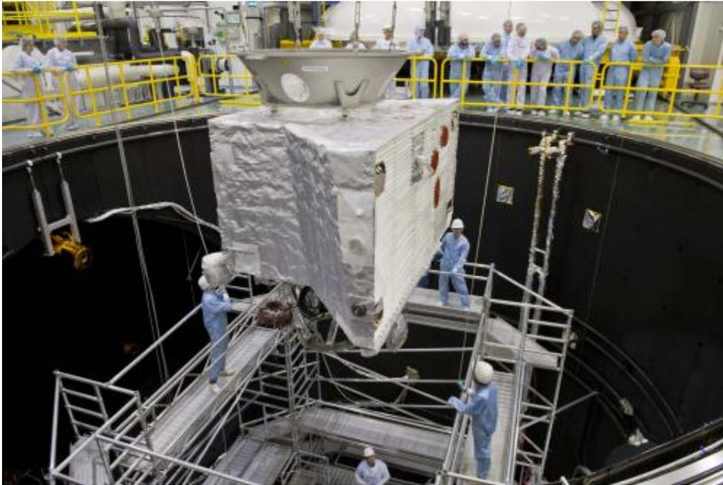
On Oct. 30, 2014, the Mercury Planetary Orbiter (part of the BepiColombo mission) was moved into the European Space Agency's space simulator for testing ahead of the expected 2016 launch. Credit: ESA–A. Le'Floch
