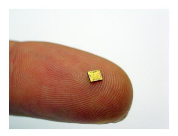
Microchip for the electrochemical detection of markers. Credit: Fraunhofer FIT
