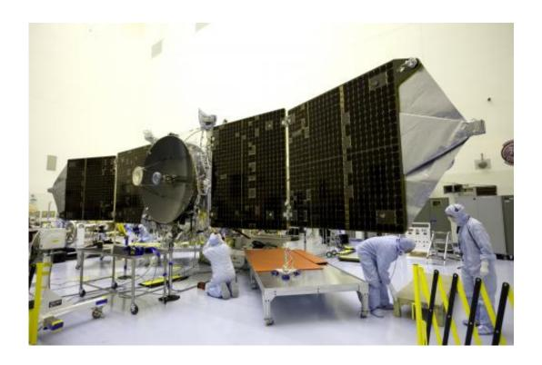
Inside the Payload Hazardous Servicing Facility at NASA's Kennedy Space Center, engineers and technicians test deploy the twin solar arrays on the Mars Atmosphere and Volatile Evolution, or MAVEN, spacecraft. Positioned in an orbit above the Red Planet, MAVEN will study the upper atmosphere of Mars in unprecedented detail. Credit: NASA/Kim Shiflett
