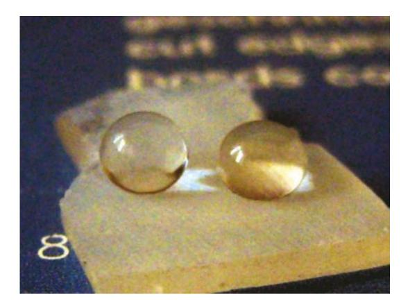
The novel material "fluoropore" repels water (left) and oil (right). These droplets do not adhere to or wet the surface. Credit: KIT/Rapp
