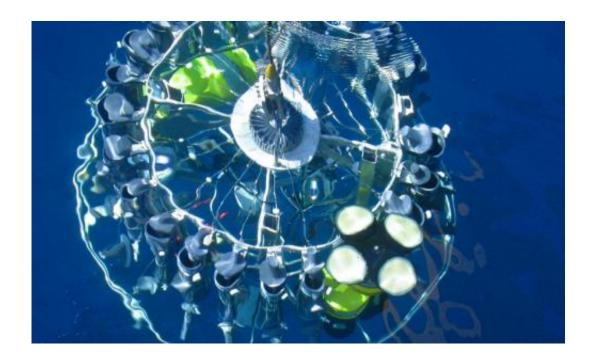
Lined with bottles triggered at different levels of the ocean, this conductivity, temperature and depth profiler bearing a suite of sampling bottles is a mainstay of oceanography. It can be deployed to depths of 6,000 meters to study changes in ocean temperature and salinity. Photo courtesy of Ann Thresher/CSIRO.
