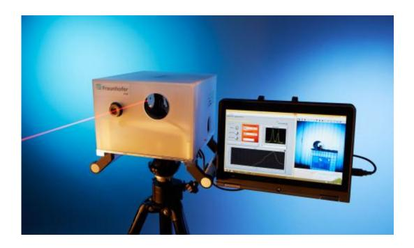
The laser-based system measures escaping biogas without contact – even from several meters away. Credit: Fraunhofer IPM
