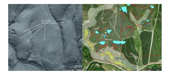
These are ancient goldmines in the Eria river valley, with channels and reservoirs for exploitation. The model generated with LiDAR data (left) allows these structures to be located on aerial photos (right). Credit: J. Fernández Lozano et al.
