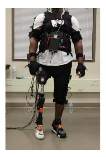
Huang's work focuses on technology that translates electrical signals in human muscle into signals that control powered prosthetic limbs. Credit: Helen Huang.
