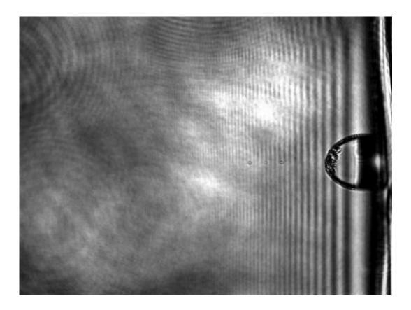
A microbullet traveling at supersonic speed is captured in this composite of three timed images as it makes its way toward a suspended sheet of multilayer graphene. Experiments carried out at Rice University show graphene is 10 times better than steel at absorbing the energy of a penetrating projectile. The bubble at left is a polymer film expanding away from the gold substrate that transfers energy from a laser to the microbullet. Credit: Thomas Research Group/Rice University
