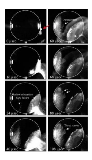
A high-speed camera recorded a laboratory simulation of colliding heavenly bodies. An analysis of shock propagation suggests what may have caused the tilted canyon-like grooves around the equator of the asteroid Vesta. Credit:
