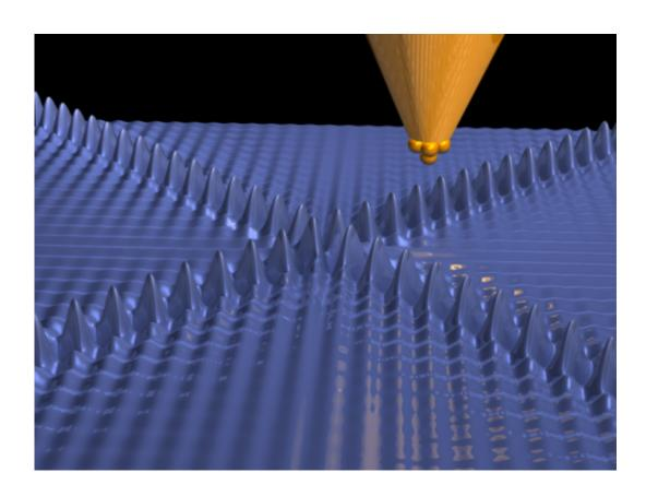
Electron density oscillations on the surface of a metallic film were made visible with the help of low temperature scanning tunneling microscopy. Credit: Forschungszentrum Jülich
