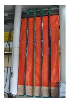
Using test setups of 6 m in height, the researchers analyze the quality of backfilling of geothermal probes. Credit: Julian Rolker/Solites
