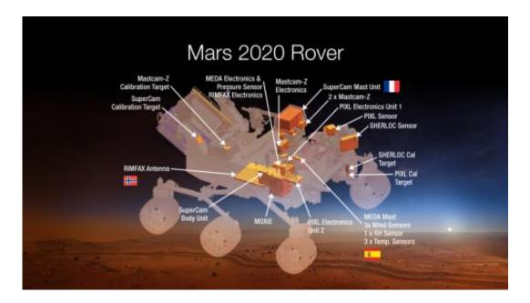
An artist concept image of where seven carefully-selected instruments will be located on NASA's Mars 2020 rover. The MOXIE payload is identified in the lower center location of the image. Credit: NASA
