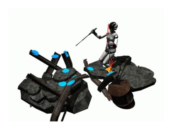
Humanoid robots have potential to use human-scale furniture, ladders, vehicles, etc. However, they still cannot negotiate disaster-like terrains. The idea of SupraPeds is to increase locomotion stability by incorporating a pair of actuated smart staffs with vision and force sensing that transforms biped humanoids into multi-legged robots. Credit: Oussama Khatib, Stanford University; Shuyun Chung, Stanford University
