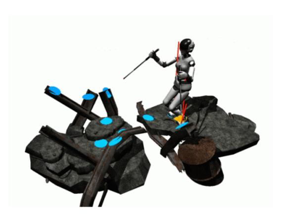
Humanoid robots have potential to use human-scale furniture, ladders, vehicles, etc. However, they still cannot negotiate disaster-like terrains. The idea of SupraPeds is to increase locomotion stability by incorporating a pair of actuated smart staffs with vision and force sensing that transforms biped humanoids into multi-legged robots. Credit: Oussama Khatib, Stanford University; Shuyun Chung, Stanford University
