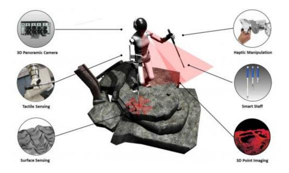
A diagram showing some of the technologies incorporated into SupraPeds' actuated smart staffs. Credit: Oussama Khatib, Stanford University; Shuyun Chung, Stanford University
