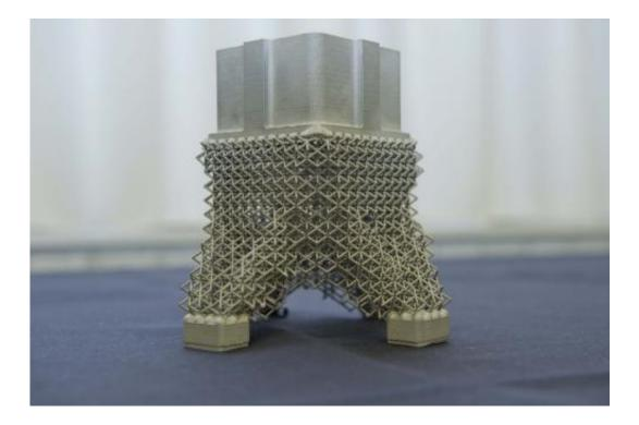
A prototype 3D-printed sensor bracket for a satellite, designed by Czech company LKE, and manufactured by Brno University of Technology. Produced through selective laser melting, this single-piece metal latticed part has reduced mass compared to its standard counterpart. Its mass is only 164 grams, compared to 222 grams for its traditionally-produced counterpart. Credit: ESA–A. Le Floc'h
