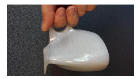
This espresso space cup was specifically designed for the low-gravity environment aboard the International Space Station.
