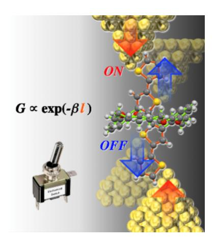
A new molecular electronic switch with three conductance states has been developed by researchers at Tokyo Tech. On-off switching is controlled by an external mechanical force.
